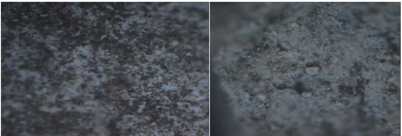
Fig. 9. Expanded Clay MgO Soaked photo 500X, a.prior to combustion b.Combustion at 800^{\circ}\text{C}
