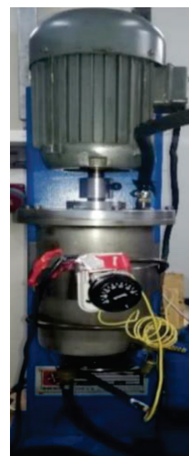
Figure 4. Electric mixer system with temperature control and fuel pump; 1 – AC motor, 2 – mixing chamber, 3 – fuel injection nozzle, 4 – fuel pump, 5 – fuel tank, 6 – heater, 7 – thermostat control, 8 – system control, 9 – blender propeller, 10 – fuel output for main tank, 11 – blender shaft, and 12 – fuel line
